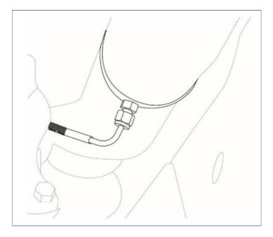
**Warning:** Installing the Exhaust Gas Temperature (EGT) Probe after the turbo may result in sub-optimal temperature feedback. To avoid this cooling effect, use the Exhaust Gas Temperature Bracket to install the EGT Probe in a pre-turbo location before the exhaust manifold. The Bracket will fit any application with an exhaust pipe that has a minimum 2 1/2" diameter and a maximum 5".
