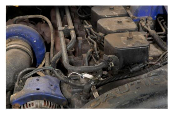
This 12 Valve Cummins Coolant Adapter allows you to install a T-Fitting for a temperature sensor on the thermostat bypass hose to read the coolant temperature of your P-Pump 12 Valve Cummins.
