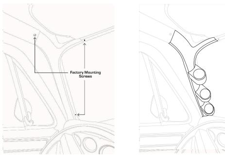
Note: This pillar pod is a complete replacement and will require removal of the factory A-pillar trim if applicable.
