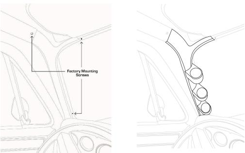
Note: This pillar pod is a complete replacement and will require removal of the factory A-pillar trim if applicable.
