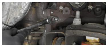
10. Loosely install the rear heat shield and tap around the ferrule fitting adapter with a hammer to make a mark on the inside of the heat shield.
