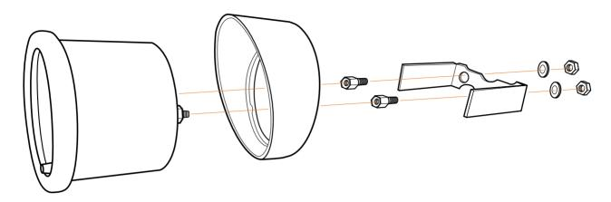
The supplied optional gauge visor is intended to be placed on the gauge so that the thickest part is at the top, creating a cover over the gauge to help keep sun glare off of the gauge face.
